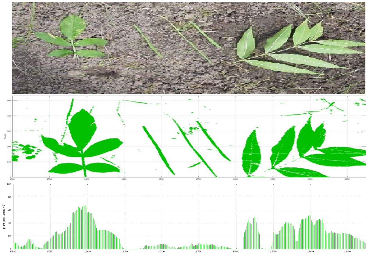
Figure 4: Measurement results for plant-soil distinction by setting corresponding trigger levels: camera signal (top), visualized output of the processed ImSpector signal (middle), weed population in percent (bottom).
