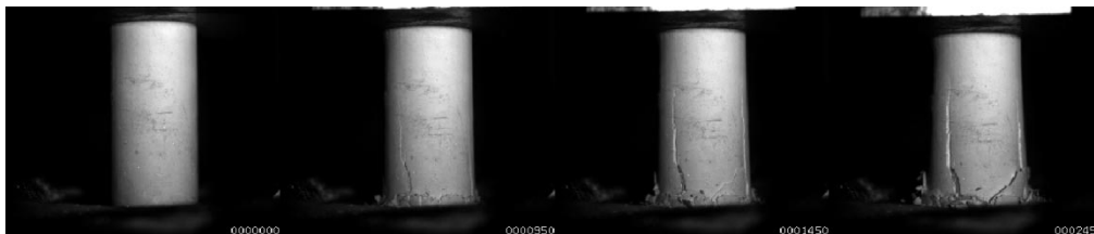
Fig. 12. Fracturing of a plaster column (frame rate: 20 000 fps).
