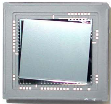
Fig. 2 A photograph of a packaged ISIS. The chip is packaged with rotation of a small angle to compensate the slanted configuration of the photodiode/pixel grid shown in Fig 1.
