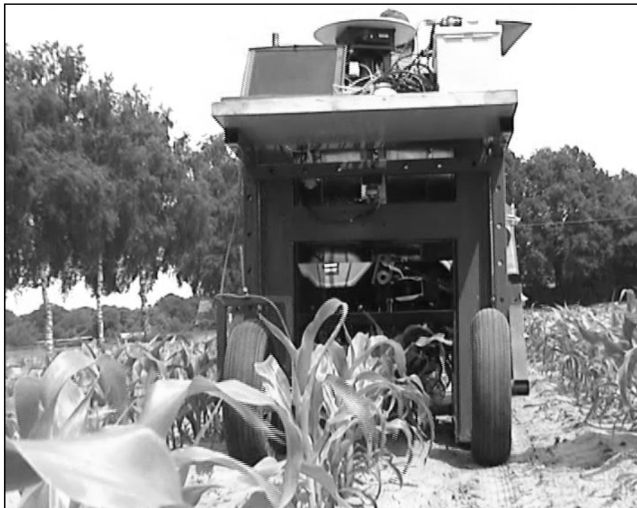
Figure 5: Sensor mobile unit with the RTK-DGPS-system in field tests.
