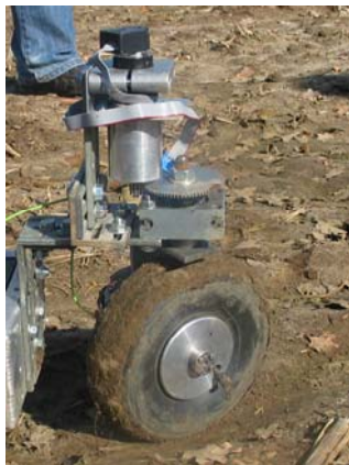
Fig. 4. Active, single steering wheel used on the FIELDMEISTER in 2006.
