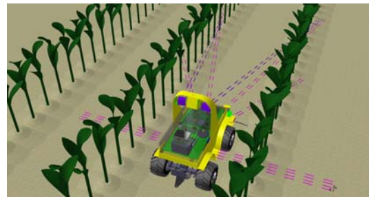
Fig. 3. MAIZERATI: Mechanical design and simulation in CATIA software.
