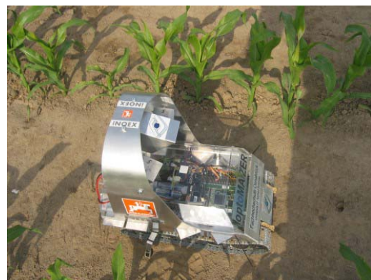
Fig 2. Field Robot OPTOMAIZER during a test run in a maize field.
