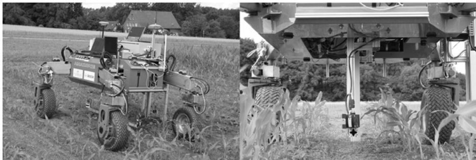
Fig. 1: The autonomous field scout “BoniRob” in field trials
