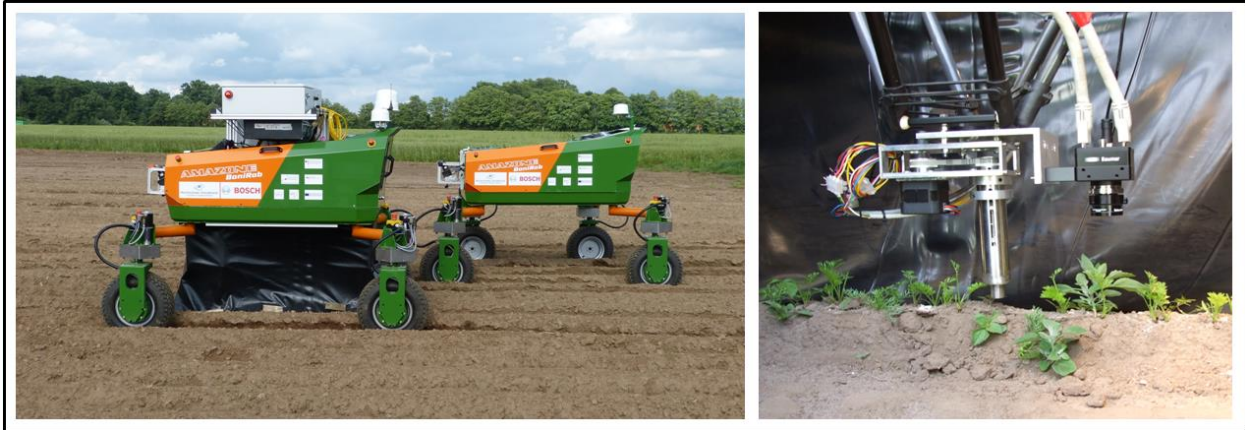
Figure 1: Autonomous field robot platform “BoniRob” with and without RemoteFarming.1 application for intra-row individual plant weed control (left). Manipulator and tube stamp actuator for single plant treatment (right)
